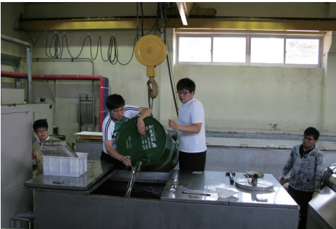
14. Increased the concentration of PEG 400 (Anjawado shipwreck)
