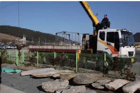
10. Gravimetric anchor stone with crane scale
