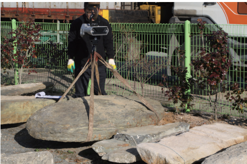
11. Gravimetric anchor stone with crane scale
