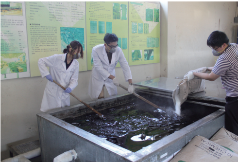
16. Increased the concentration of PEG 4000 (Anjawado shipwreck)
