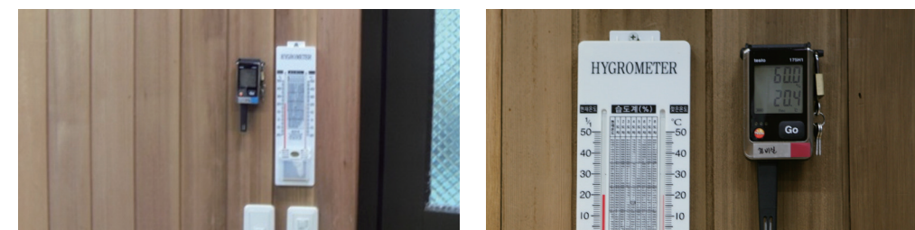
1, 2. Temperature and humidity monitoring (Testo 175H1, Humidity and Temperature data logger) in the storage
