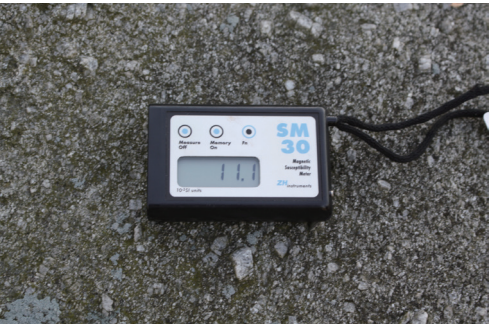
12. Measurement of whole-rock magnetic susceptibility rate
