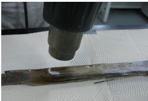
59. Surface treatment using heat-gun
